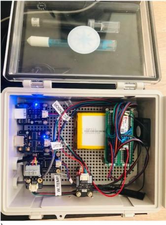
The xElectron can be customized to include a specific sensor that I available on the market e.g. ,Water Turbidity, Dissolved Oxygen, ORP, Anemometer, etc.
